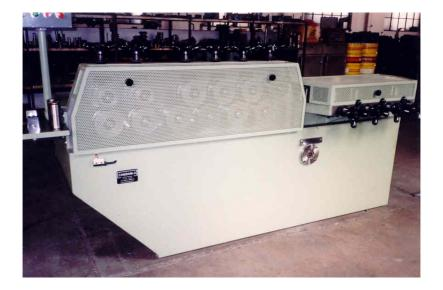
Straightening and cutting machine for the production of bars with many different section shapes (square, rctangular, hexagonal, ecc...)
