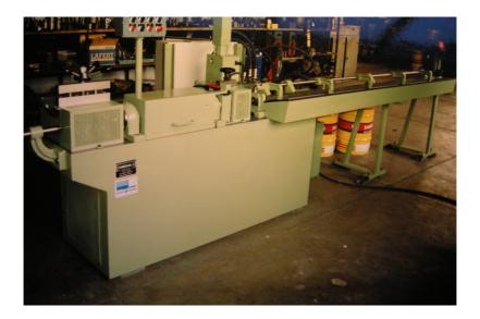
Straightening and cutting machine with straightening bushes 1 o 2 Inverter can control the straightening frame rotational speed and the wire feeding speed
