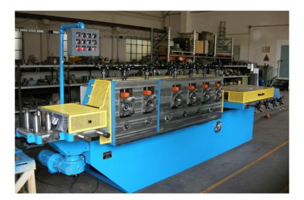
Straightening machine for the production of bars with many different section shapes (square, rectangular, hexagonal, ecc...)
