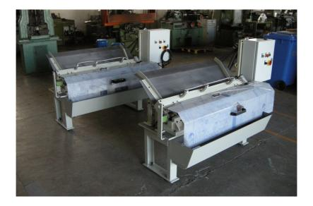
Pressing unit for rod stamping, to apply to existing straightening machines
